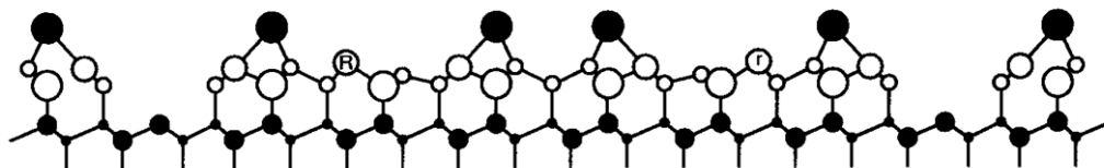
Fig. 2.26. Side view of the surface structure of the DAS model of the Si(111)-(7 × 7) surface (Takayanagi et al., 1985b).
